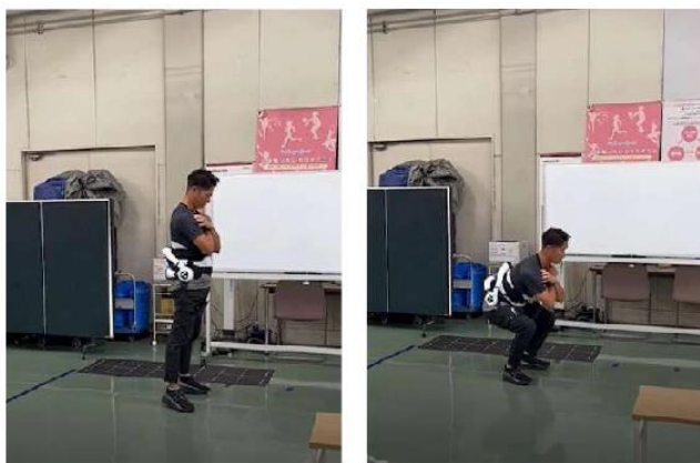
Figure 5. CVC squat exercise with the Hybrid Assistive Limb.
