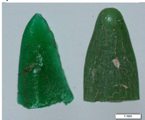
Fig.7-4 Comparison of green spatula MP immediately after breaking and after drifting ashore. The left is scattered fragment on the street and the right is beached fragment on the coast. Scale bar represents 1 mm.
