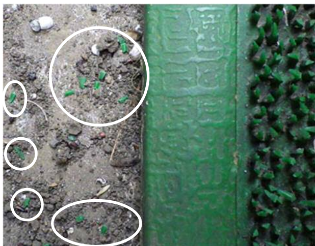
Fig.7-3 Status of the entrance mat where the protrusions were broken. Fragments of protrusions is scattered in the white circle.
