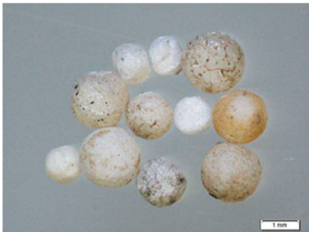
Fig.3-1 Beached PS spherules on the coast. Sampling point of these spherules was Sanno-Ami-Issiki. Scale bar represents 1 mm.
