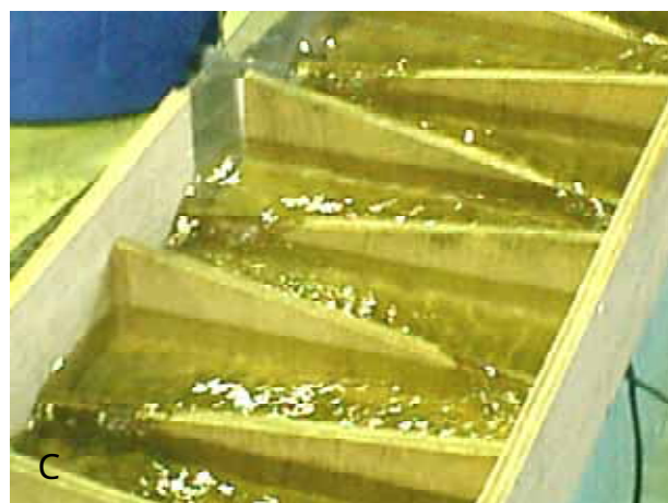
Fig.1 Structure of an experimental equipment, A a Fishway equipment ; B Cascade-M type ; C Chidori-X type
